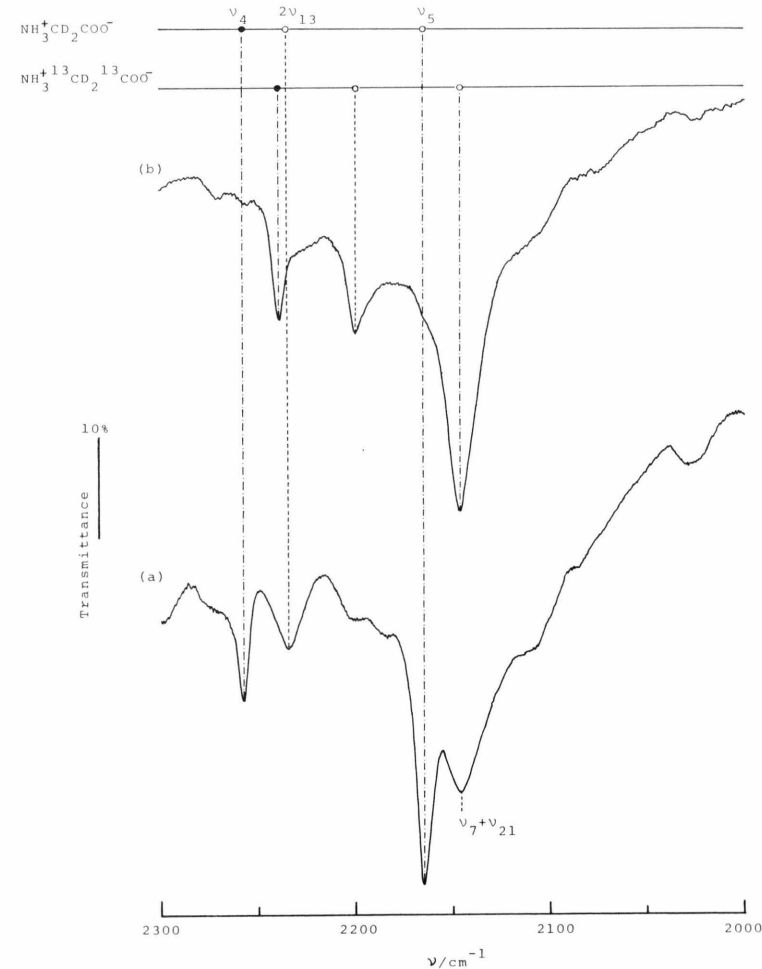
Fig.4. Characteristic absorption bands due to C—D stretching modes of \alpha -NH 3 + CD 2 COO - (a) and \alpha -NH 3 + 13 CD 2 13 COO - (b) at 80 K. The final assignments for fundamentals are indicated as symbols \nu_i at the top of the spectra.
